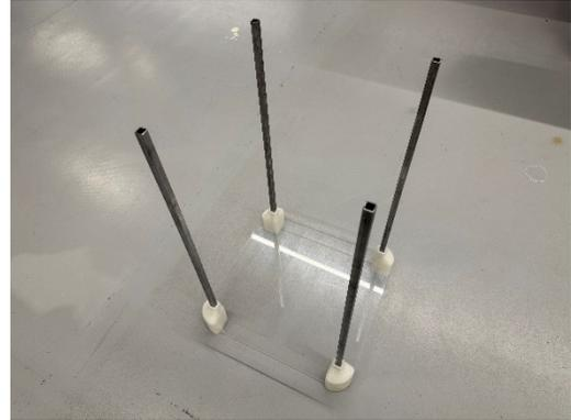
6. Notice that one of the 3D-printed stands for the upper main plate has a slot for a set of M6 nuts and washers. These can be secured by friction. Unlike the printed parts for the base plate, these parts are secured onto the main plate using M3 screws and washers.
