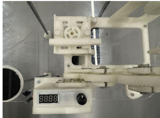
13. Install the 4 x M6 540mm threaded rods with M6 nuts and washers. These M6 rods are positioned around the top-left hand side. For individuals working on this project, installing M6 nuts on both ends could help stabilize the structure.
