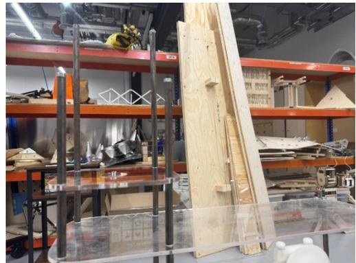
20. Install the extruder controller and the 2 x 45mm steel tubes. After that, install the extruder motor acrylic plate. Next, install the 3D printed extruder stand on to the acrylic plate. Tighten all the nuts when you are done.
