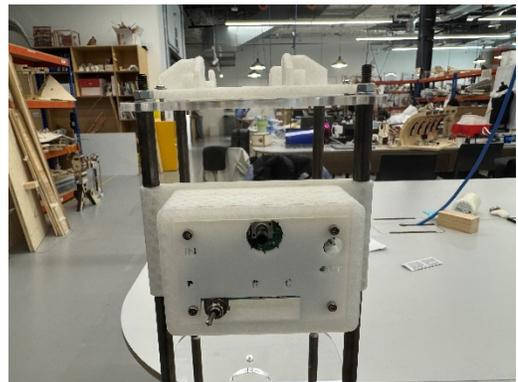
21. Carefully place the extruder onto the extruder stand. The motor should be pointing towards the left-hand side of the installation. Screw the plastic nuts and washers onto the 6mm threads that comes with the extruder.
