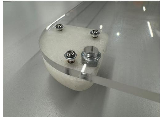
7. The main acrylic plate is then slotted in onto four of the square steel rods.
