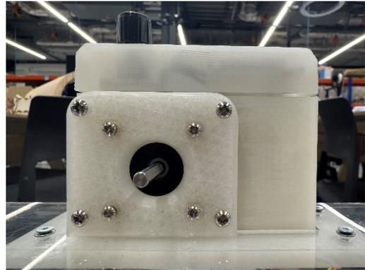
11. Install the large attachment plate with 4 x M3 screws. Before installing, check all the wires are properly secured. This can be accomplished with soft silicone tape. Make sure the tape is non-conductive. The wires should all run through the bottom hole of the controller. The motor controller is now complete; it should be sitting flush against the edge of the table.
