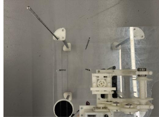
14. Similarly, install the 2 x M6 240mm threaded rods with M6 nuts and washers around the right-hand side of the main acrylic board.
